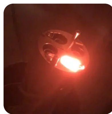
Figure 1: Evap-4 mounted inside the PVD chamber with pocket 3 powered up.
